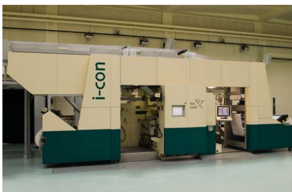
KBA-GIORI's i-con web-fed intaglio system for tax stamps and other non-currency high security documents
